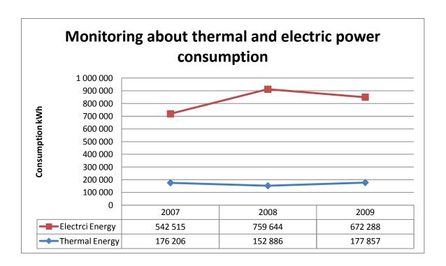
ASP L.Martelli has an important heat loss due to the age of the building and no insulation layer inside the external walls. This RCHEP will implement solar thermal and automatic thermal regulation system to reduce its energy consumption.
